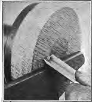
Fig. 271. Turning the Face with Roughing Gouge.
